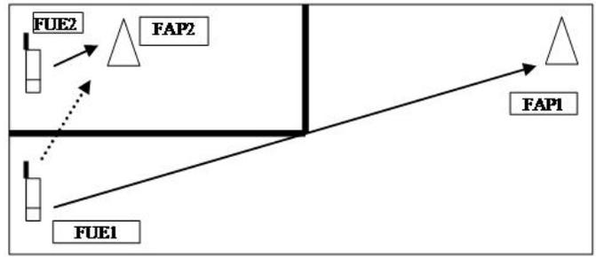
Fig. 1. Femtocell-to-Femtocell Uplink Attack
