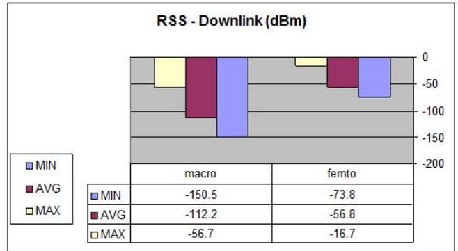
Fig. 5. RSS in Downlink with concentration at the edge
