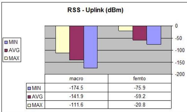
Fig. 8. RSS in Uplink with concentration in the center
