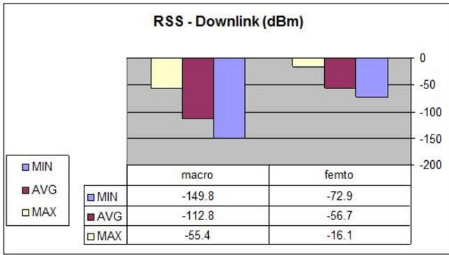
Fig. 3. RSS in Downlink with uniform distribution
