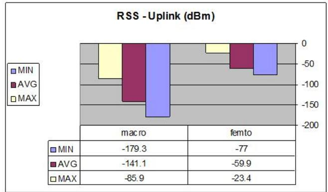
Fig. 4. RSS in Uplink with uniform distribution
