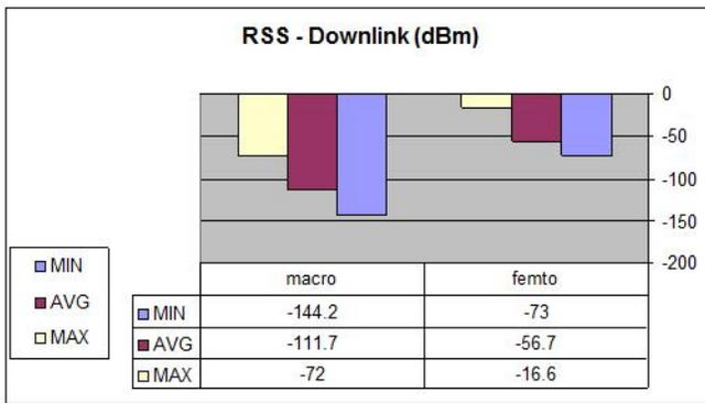
Fig. 7. RSS in Downlink with concentration in the center
