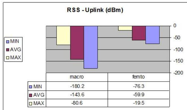
Fig. 6. RSS in Uplink with concentration at the edge
