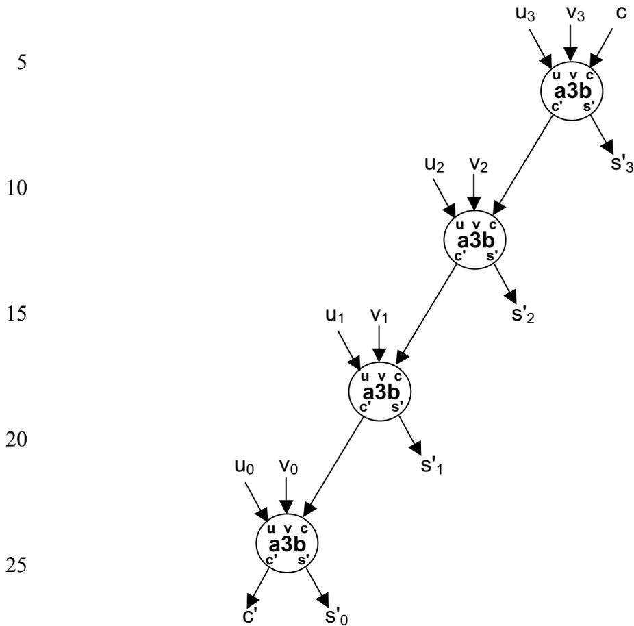
30 Note that this diagram represents a circuit for a serial adder, and this was obtained from the flexible algorithm by a process called symbolic execution, which is similar to the usual execution. Similar diagrams may be found in introductory books on digital logic and systems.
